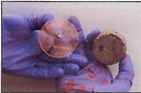
Figure 2. Examples of PVC (left) and concrete (right) coupons
