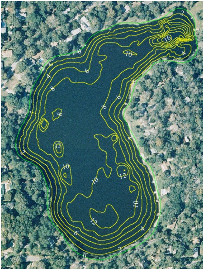
Figure 2-1. Depth Contour Map for Lake Florida (Source: Seminole County Water Resource Atlas)
