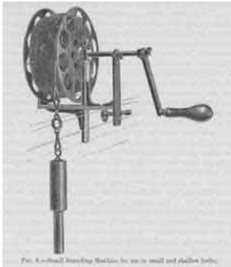
Sounding machine developed circa 1895, consisting of a take-up reel and handle. The sounding weight is suspended from the reel. (Murray and Pullar, 1910, Fig. 6, p. 13). Courtesy of the National Library of Scotland - www.nls.uk .
